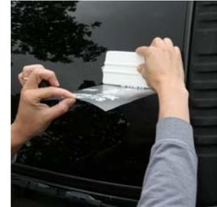
\* For larger decals, using the squeegee, work the decal down starting at the middle and working your way out. Once you have applied the right side of the decal, remove the masking tape and peel the left side back to repeat the process.
